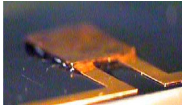
Figure 2. Embedded thermoelectric cooler, with total height of 100 microns and 2.5 \text{ mm} \times 2.5 \text{ mm} footprint
